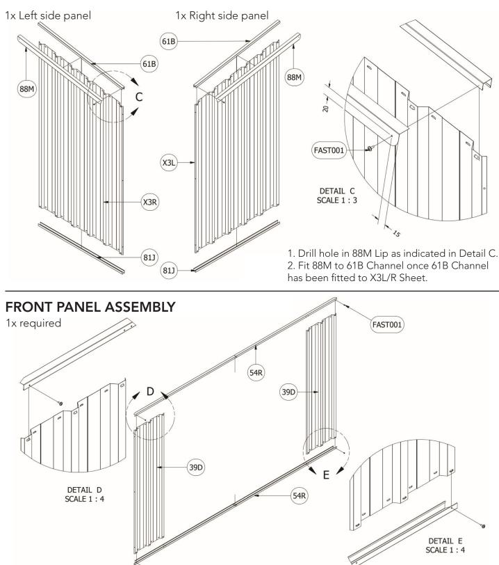
The FAST001 screws illustrated in this process locate the 54R channels onto the sheets in an important position which will determine correct alignment of the doors and lid. It is important that these are installed before proceeding further.
