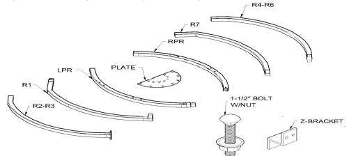
**Step 2:** Connect R1 And R7, and Connect LPR and RPR. You may need a rubber mallet to set the tubing into the fittings.
