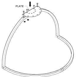
**Step 5:** Attach R2, R3, R4, R5, R6 to top plate. Use self tapping screws to secure the ribs to LPR and RPR.
