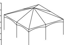
**1.** The layout begins with the frame parts being laid out on the ground in the approximate location that they will be when the frame is assembled. The perimeter parts are laid out to form the perimeter, and the roof support parts are placed in the interior in their general locations. Laying out the parts in this way facilitates the assembly. (See Diagram)
