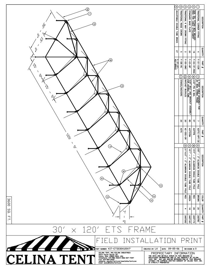
**1.** A minimum of 8 people and 5 frame tent jacks are recommended for the proper installation of this tent. Refer to the parts list at the top of the diagram to make sure you received all parts required for proper installation of this tent.
