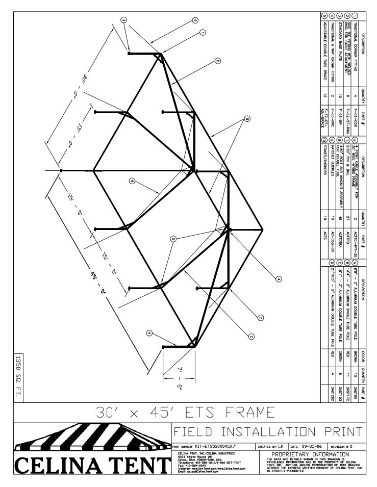
**1.** A minimum of 6 people and 2 frame tent jacks are recommended for the proper installation of this tent. Refer to the parts list at the top of the diagram to make sure you received all parts required for proper installation of this tent.
