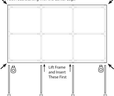
6) Lift the Opposite Side of the Canopy and Attach the Legs and Foot Pads in Same Way. Begin with the Center Legs.
