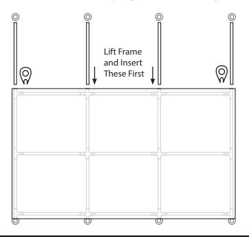
7) Attach the Side Walls with the Straps to the Frame on Both Sides, then Attach the Valance Straps to the Center Legs and Hook on to the Foot Pads and Tighten. Lastly, Fasten the Drawstring to the C-Clip at Each Corner and Tighten by Pulling the Cord Down and Hooking it into the Clip. Secure the Flaps on the Side Walls by Wrapping Them Around the Outside of Pole and Attaching to the End Walls.
