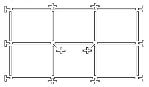
2) Assemble Frame Starting with Center Ridge.
