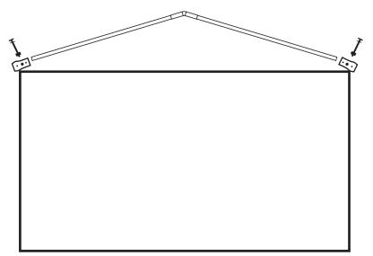
3) Add Center Ridge Section and Complete the Frame Setup by Repeating
