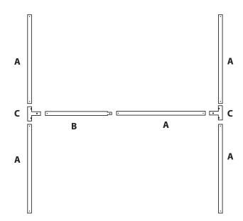
2) Assemble One End of A Frame by Attaching Clamps on Both Sides to Kennel Cage and Insert Pipes and Fitting as Shown Below.
