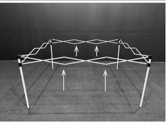
3) Open Frame by Pulling it Apart at the Center of the Lower Truss Bars. Do this by Standing On Opposite Sides and Walking Back While Pulling Frame Open. Snap Corner Lock Fittings into Place by Pushing Slider Fitting Up While Holding Top Corner Down with Your Other Hand.
