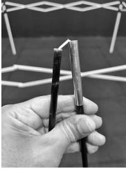
4) Assemble the Roof Rods by Inserting One Into the Other at the Corded Joints.
