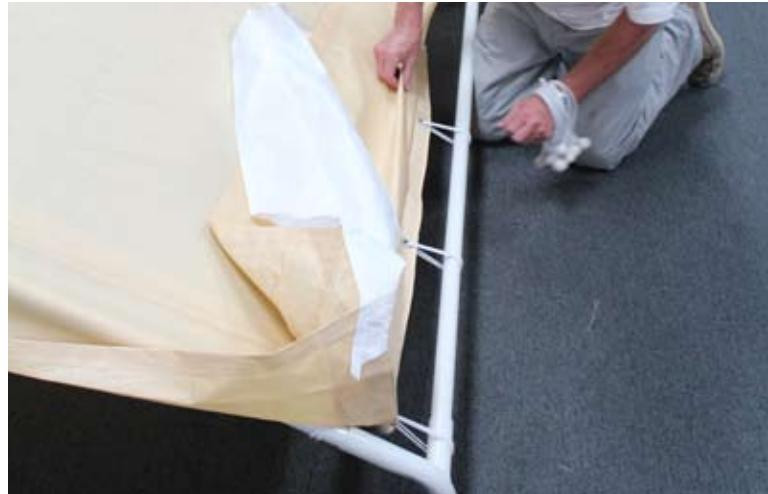
**7)** Next continue attaching the straps down each side and end. Make sure the cover stays centered on the frame.
