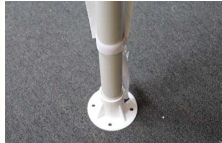
**12)** Secure the hook and loop straps on the cover at all 4 corners around the corner 3-way fittings.
