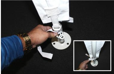
11) Attach each D-ring at each foot pad and pull to tighten. If screens will not be used you can go ahead and attach hook and loop strap around the leg also. If the screens will be installed wait to attach the D-ring until after the screen has been tied to the 4-way fitting to make attachment process easier.
