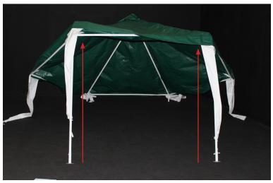
**8)** Lift frame on one side and insert 2 legs as shown. Make sure thumb buttons snap into the 4-way fitting to lock leg in place.
