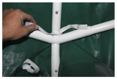
**12)** Position each screen section around the outside of the leg and tie the strap around the top of the 4-way fitting to hold wall in place.
