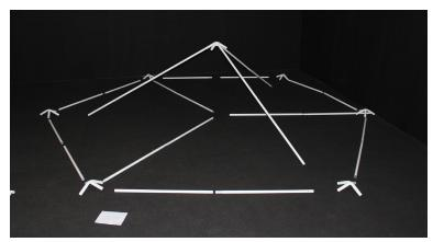
**2)** Begin connecting the center peak fitting to the peak pipes. Align the thumb buttons to the holes in the fitting until they snap in place. Form a tripod by skipping a section so that you can get the frame to stand as shown above .
