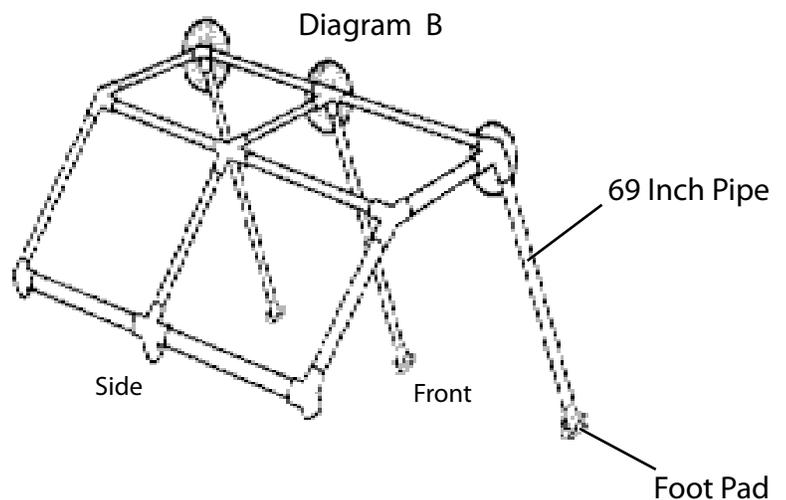
**3-** With the top frame laying over on one side and the legs inserted on the other side as seen in Diagram B, drape the one piece cover with sides and rear wall over the frame. Make sure you have the open end in the direction needed. Pull the one side down over the frame with the legs inserted. You can also pull the rear over the frame partially. Next, insert the legs on the opposite side and pull the remainder of the cover on.
