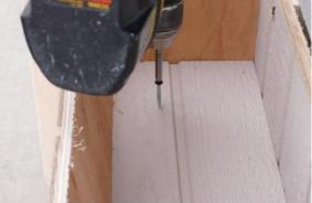
Fasten with 1 1/4" black headed screws into the mount as well.
