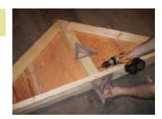
Then fasten panels L and M together. Be sure to keep even as shown.
