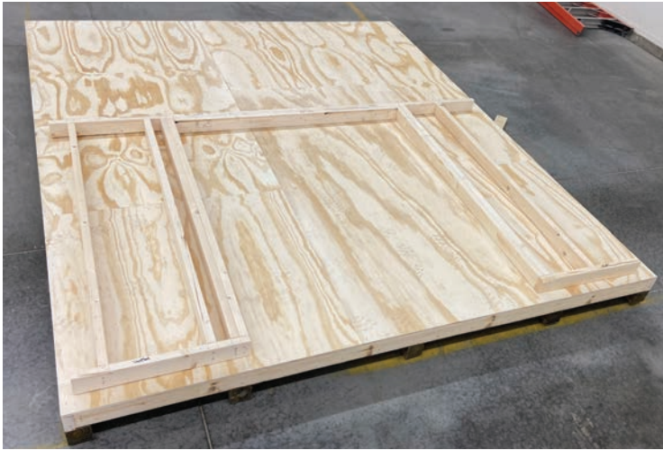
19. Completed Door Framing.
