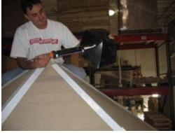
You will find a cut in the cap. Insert a bead of caulk before installing.
