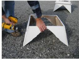
As you construct the pieces together you will want to install 2, 1 1/4" block head screws into each corner.
