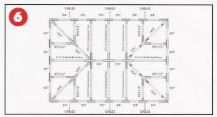
Finally, attach cross support cables across the center to the mid-leg rafter fitting. Then attach appropriate anchoring and secure cover tightly with straps & buckles.
