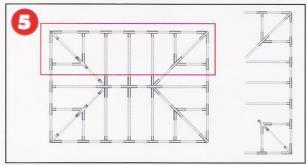
With the cover on the frame loosely, add legs on to the longer side and then do the same the opposite side. Last, put in the remainder of the legs.
