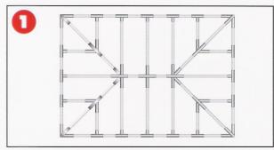
Lay out tubing on a flat surface based on the frame sketch provided. (Example: 40' x 60')
