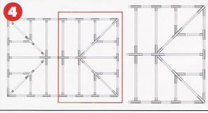
Add Mid Truss Double Tube and attach to the 4-Way Top Expansion Fitting. Then add Top Bar and connect to the 6-Way Crown. Continue until tent is complete.
