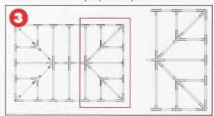
Complete both ends including Double Tube Trusses to the 6-way Top Fitting (8-Way Top Fitting on a 40'x 40'). When top portion of frame is complete and still on the ground, place cover on loosely over frame. If expandable, do the lacing once both ends are in place.
