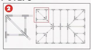
Make all four  $\frac{1}{2}$  corners to the Y-Fitting and then add corner cables.
