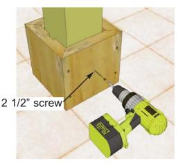
**25.** With your helpers assistance, screw Part J & K pieces together with 2 - 2" screws at pre-drilled locations. Make sure pieces are aligned on edges and top and bottom. Cleated skirting piece are pre-drilled. Complete remaining skirting pieces around the post. Position skirting unit evenly around post. Secure to post by screwing 1 - 2 1/2" screw into the center of each cleated skirting piece (J).
