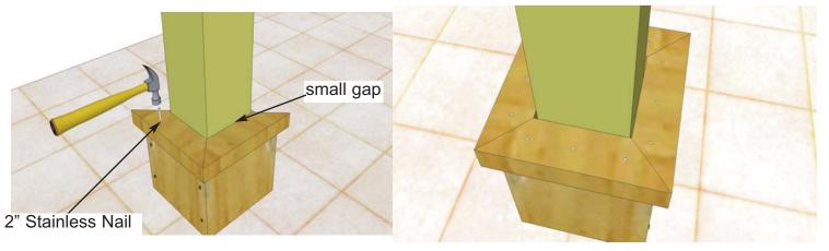
**26.** Position **Post Skirting Caps - 1 1/2"** x **2 1/2"** x **10 5/8"** (**Part L**) on top of skirting unit and against post. Do a dry run first to confirm fit. There will be a small gap between post and inside of cap. Attach caps down into skirting tops with **3 - 2" Stainless Steel Finishing Nails** per piece. Complete remaining post skirtings.
