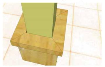
**26.** Position **Post Skirting Caps - 1 1/2"** x **2 1/2"** x **10 5/8"** (L) on top of skirting unit and against post. **Dry fit pieces first to confirm proper fit.** There will be a small gap between post and inside of cap. Attach caps down into skirting tops with **3 - 2 1/2" Stainless Steel Finishing Nails** per piece. Complete remaining post skirtings.
