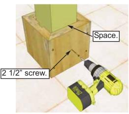
**25.** With your helper's assistance, screw Parts J & K pieces together with **2 - 2" screws** at pre-drilled locations. Make sure pieces are aligned on edges and top and bottom. Cleated skirting pieces are pre-drilled. Complete remaining skirting pieces around the Post. Center skirting kit evenly around Post. Secure to post by screwing **1 - 2 1/2" screw** into the center of each Cleated Skirting Piece (J).
