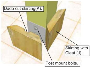
**24.** Locate all Post Skirting pieces. Position 2 post skirtings around the base of post as shown above. Use 1 Post Skirting with Cleat - 1 1/2" x 9" x 10" (J) and a Post Skirting with Dado Cut - 1 1/2" x 9" x 10" (K) initially. Cleated piece should be aligned opposite post mount hardware and dado piece aligned with post mount bolts (hardware).
