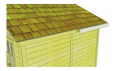
**62.** Attach **Side Facia** to roof rafter ends. There are 2 Facia pieces per side. Secure with 6 - 1 1/2" finishing nails per piece.
