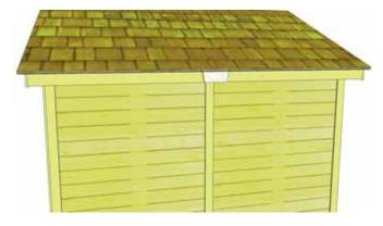
**66.** Attach Horizontal Gable Trim Detail and Facia Trim Detail Plates to cover seams where facia and horizontal trim pieces come together. Horizontal Gable Trim Detail Plates are 4 1/2" high while Facia Trim Detail Plates are 3 1/2" high. Secure each with 4 - 1 1/2" finishing nails per piece.
