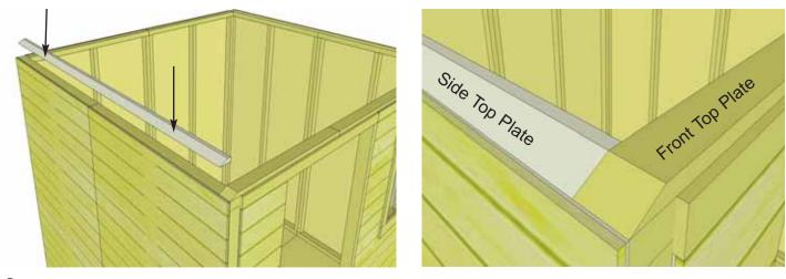
**29.** Next, attach the 2 **Side Top Plates** (1 per side). The side top plates are angle cut down the Edge. Once again, position top plate on wall plate so it is flush with inside of wall framing. Side plate should also be flush with Front Top Plate. Secure with 4 - 2" screws per piece.
