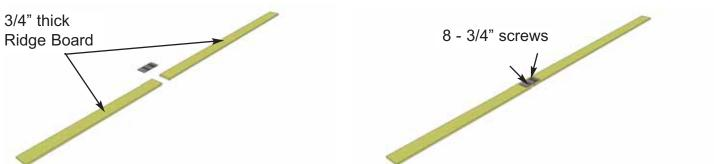
**35.** Locate 3/4" x 4 1/2" x **57 1/2" & 33 1/2" Ridge Boards** and attach together with **Metal Ridge Board Connector** using 8 - 3/4" screws. Total Length when connected is 91". Complete two Sets. Position Metal Ridge Board Connector evenly on Ridge Boards.
