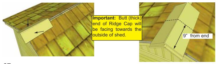
**67.** Place First Roof Ridge Cap on roof peak overhanging shingles by approximately 2". Attach with 2- 1 1/2" Shingle Nails 9" from end. Place 2nd Ridge Cap 1" back from 1st cap. Attach with 2- 1 1/2" Shingle Nails 9" from end.
