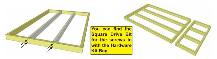
2. When correctly positioned, attach each Joist with 4 - 2 1/2" screws (2 per end).
