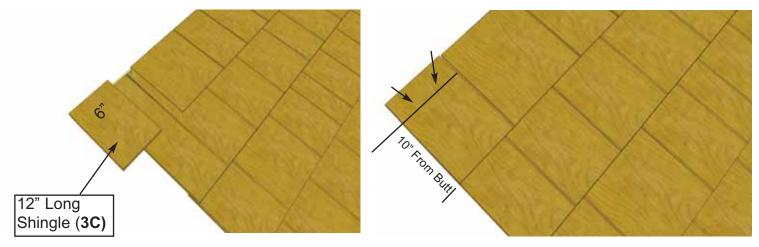
**24.** To finish end, place and attach (**3C**) shingle (6" wide x 12" long) in line with 5th and final row of shingles. Shingle (**3C**) will partially cover shingle (**3B**). Secure with **2 - 7/8" Shingle Nails (M)** 10" from butt.
