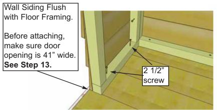
**12.** Align butt or bottom of wall siding flush with outside of floor framing. When correctly positioned, secure bottom wall plate to floor with **2 - 2 1/2" Screws (C)**. Attach vertical wall framings together at top, middle and bottom with **3 - 2 1/2" Screws (C)**.
