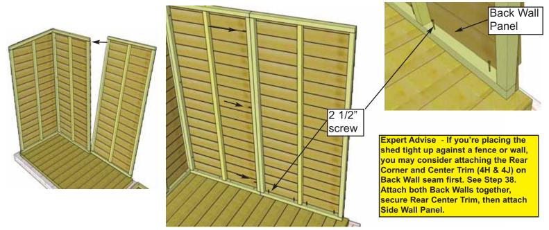
**9.** Position 2nd **Back Wall Panel (2C)** on Floor as per **Step 8**. Attach wall frames together at top, middle and bottom with 3 - 2 1/2" screws. Secure bottom wall plate to floor with **4 - 2 1/2**" **Screws (C)**.
