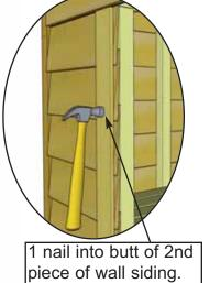
**30.** Locate 2 **Vertical Door Frame Trims (4C) (1/2" x 2 1/2" x 64 1/4").** Position on front narrow wall flush with outside of wall framing and tight underneath front horizontal trim. Attach with **1 - 1 1/2" Finishing Nail (K)** on second piece of wall siding into the butt (where trim and siding touch).
