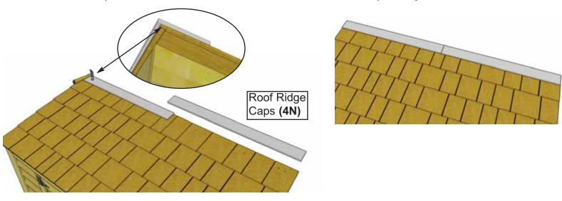
**43** Using a Step Ladder, place both **Roof Ridge Caps (4N) (1/2" x 3 1/2" x 39")** on rear row of roof shingles. Ridge Caps will overhang shingles by 1/4". Attach each piece with **4 - 1 1/2" Finishing Nails (K).**
