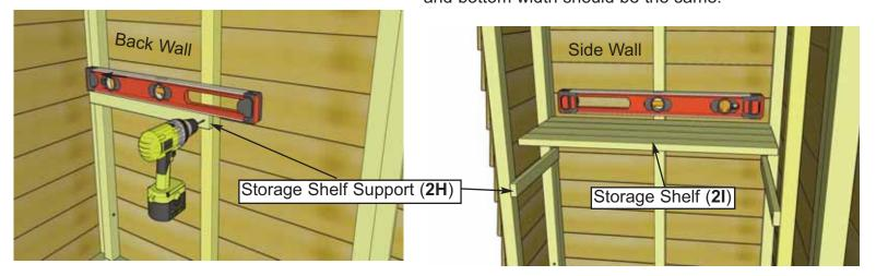
**18.** Storage Shelf positioning is flexible so decide what height configuration suits your needs. Gather your **Storage Shelf Supports (2H)**. The short Support (14 1/2") attaches to the narrow wall, the long (18 1/4") to the back wall. Position using a Level, and drill Pilot Holes to prevent ends of Supports from splitting. Attach first Support using **2 - 1 1/4" Screws (E)**. Place Storage Shelf on attached Support, Level, and mark position of 2nd Support. Pilot Hole and secure 2nd Support.
