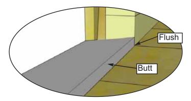
32. Locate Door Threshold (4Q) (1/2"thick at butt x 2 5/8" wide x 40 7/8"). Position threshold on floor in the opening. Align with thick side of the bevel to the inside flush with the wall stud. Attach with 4 - 1 1/4" Screws (E).
