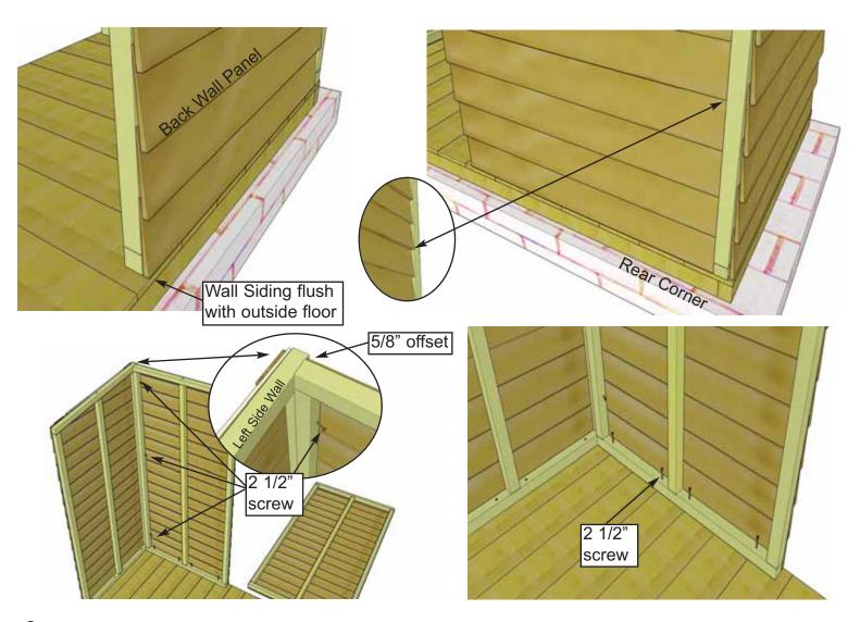
8. When side and back walls are aligned in corner correctly, wall framings will be offset. Screw wall framings together with 3 - 2 1/2" Screws (C). Secure bottom wall plate to floor with 4 - 2 1/2" screws (C).
