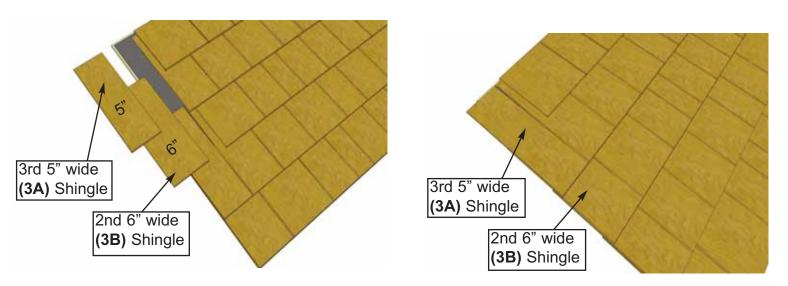
**23.** Place and attach 2nd (**3B**) Shingle (6" wide) in line with 3rd row of shingles. Shingle (**3B**) will partially cover shingle (**3A**). Secure with **2 - 7/8" Shingle Nails (M)** 8" from Butt. Complete attachment of 3rd 5" wide (**3A**) shingle.
