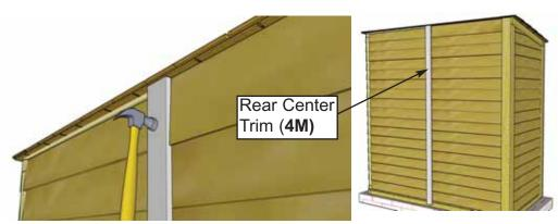
41. Locate Rear Center Trim (4M) (1/2" x 2 1/2" x 72"). Align tight against upper rear trim and underneath roof. Attach with 6 - 1 1/2" Finishing Nails (K).
