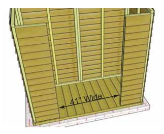
**13.** Align and attach the second front narrow wall panel as per **Step 12**.
