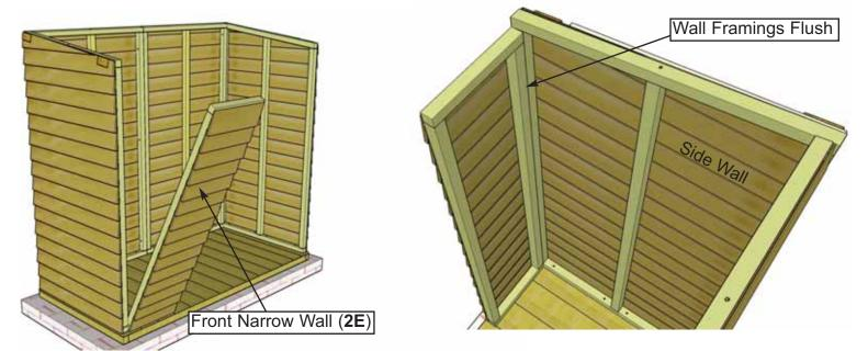
**11.** Locate **Front Narrow Walls (2E)** and position wall framing flush with side wall framing in corner. Make sure narrow wall is positioned right side up.
