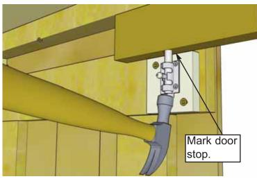
**49.** Position the **Interior Silver Barrel Bolt (BB)** on the plywood spacer and attach with **4 - 3/4" Silver Screws (G).** Tap barrel bolt with hammer on underside of interior door stop to mark location.
