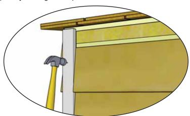
28. Locate 2 Front Filler Trims (4A) (1 1/2" x 5/8" x 65"). Filler trim will be covered by corner trim in Step 37. Attach in each front corner with 6 - 1 1/2" Finishing Nails (K).
