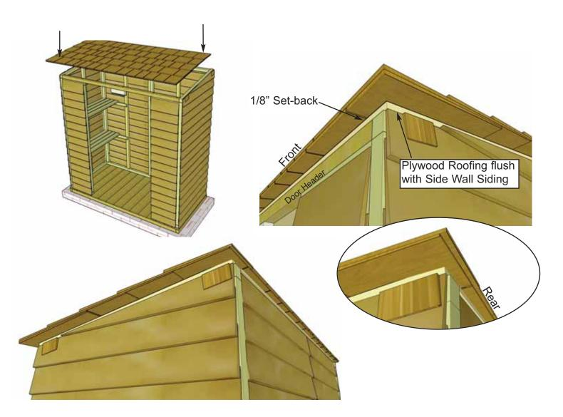
**26.** Lift up completed cedar shingle roof panel and place on upper wall framing. In the front, align plywood roofing 1/8" back from door header. On the side, plywood should be flush with side wall siding. Equally space roof from side-to-side. In the rear, plywood should sit on back wall top plate.
