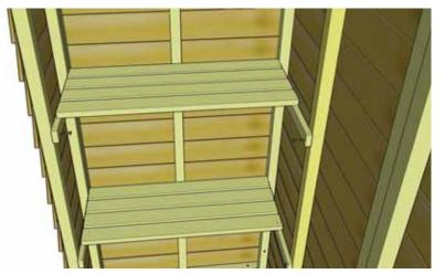
19. Place Storage Shelf (2I) on top of supports and secure with 4 - 1 1/2" Finishing Nails (K). Complete 2nd Shelf (if desired) as per Steps 18 & 19.
