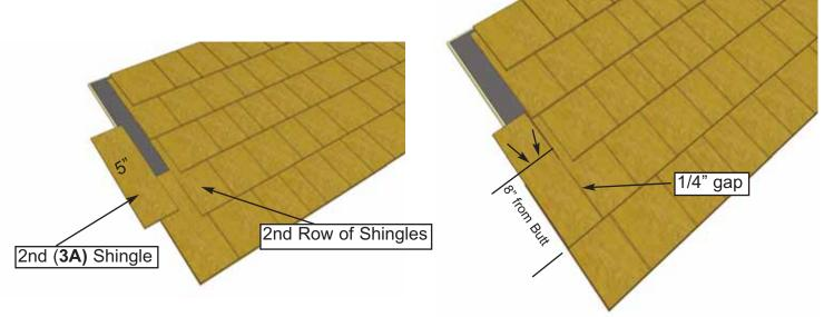
**22.** Place and attach second (**3A**) Shingle (5" wide) in line with 2nd row of shingles. Shingle (**3A**) will partially cover shingle (**3B**). Secure with **2 - 7/8" Shingle Nails (M)** 8" from butt.
