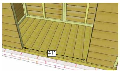
**17.** When all walls are attached together, check door width at top and bottom. Door width should be 41" wide. If required, loosen narrow and side wall plate screws, adjust door width and re-secure. There can be an 1/8" tolerance in the width but top and bottom width should be the same.
