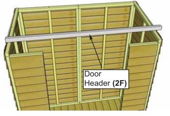
**14.** Locate **Door Header (2F) (1 1/2" x 1 1/2" x 70")** and place on top of front narrow wall framings.
