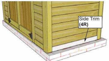
45. Attach both Lower Side Narrow Trims (4R) (1/2" x 2 1/2" x 33 1/8"). Place trims between front and rear corner trims to cover part of floor frame with 4 - 1 1/2" Finishing Nails (K).
