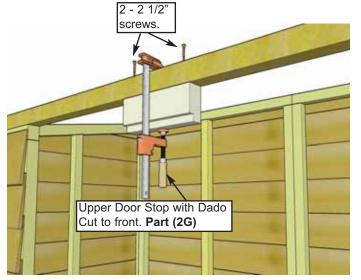
**16.** Attach **Upper Door Stop (2G).** Dado cut aligned to the front. Center on door header and attach with **2 - 2 1/2" Screws (C)**. Screw down from the header into Stop. Use Clamp to hold stop.
