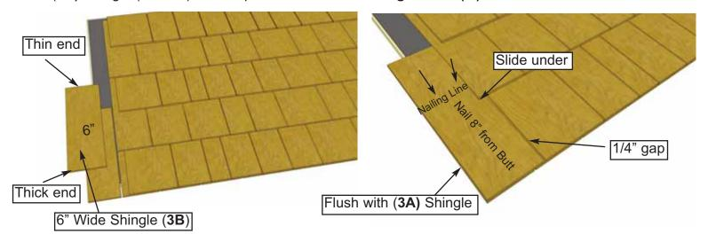
**21.** Place and attach (**3B**) Shingle (6" wide) directly on top of Shingle (**3A**). Shingle (**3B**) will slide under 2nd row shingle. Secure with **2 - 7/8" Shingle Nails (M)** 8" from butt.
