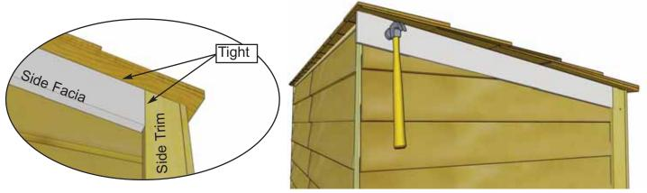
**39.** Continuing around the shed, place a **Side Facia Trim (4I) angle cut both ends (1/2" x 2 1/2" x 33 7/8")** tight against front side corner trim and snug underneath roof panel. Attach side facia into side wall cleats with **4 - 1 1/2" Finishing Nails (K).**
