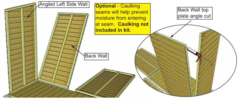
7. With your helper holding the side wall panel, position a Back Wall Panel (2C) in rear corner. Important: Align Wall Siding Flush with Floor Framing.
