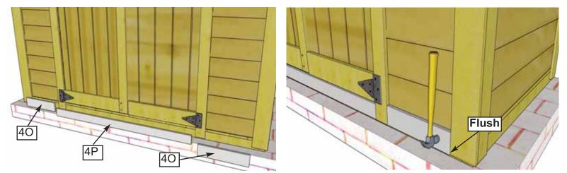
**44.** Locate both **Lower Front Narrow Trims (40) (1/2" x 2 1/2" x 11 1/8") and Doorway Narrow Trim (4P) (1/2" x 2" x 40 7/8").** Place narrow wall trims between door trim and front corner trim flush with bottom of trims. Attach each with **2 - 1 1/2" Finishing Nails.** Place lower door trim between door trims flush with bottom. Attach with **4 - 1 1/2" Finishing Nails (K).**
