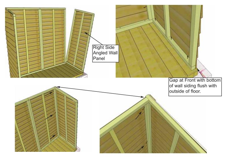
10. In the corner, align and attach right Side Wall (2A) framing to back wall framing as per Steps 7 & 8. Secure bottom wall plate of side wall to floor with 4 - 2 1/2" Screws (C).
