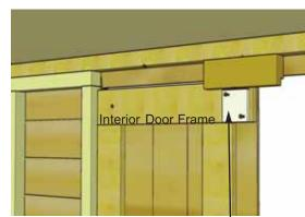
**48.** Install the Barrel Bolt Plywood Spacer (UU) to interior door frame, flush at the bottom, and 1/4" from edge, as pictured. Use 2 - 1 1/4" Screws (E) to secure.
