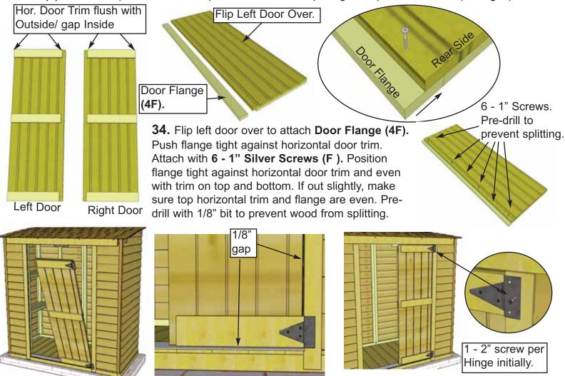
**35.** Starting with right door first, lift and position door in opening. Leave a 1/8" gap on right side and 1/8" gap on the bottom. Use a **Shim Shingle (4T)** to shim the door at bottom to help position door evenly. When door is aligned correctly, screw hinge into vertical door frame trim with **1 - 2" Black Headed Screws (H).** Use only 1 screw initially per hinge until both door alignments are confirmed. Drill pilot holes to prevent wood from splitting.
