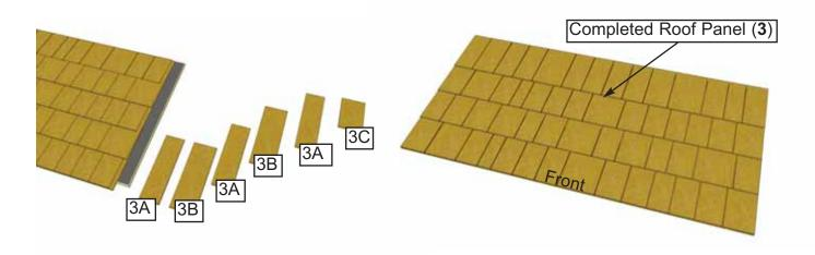
25. Complete attachment of shingles on opposite side of roof panel following Steps 20-24.
