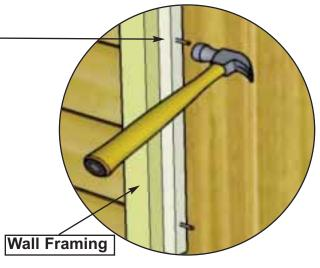
**51.** Attach Interior Vertical Interior Door Stops (4S) (3/4" x 3/4" x 31 5/8" x 4 pcs.) to inside wall framing with 4 - 1 1/2" Finishing Nails (K) per piece. To align correctly, close door to make sure stops are close to the door but don't interfer with their closing. Attach bottom piece first with hammer.
