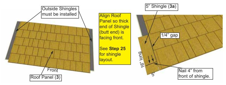
**20.** Lay **Roof Panel (3)** on flat level ground. Note, overhanging Outside Shingles have been removed to avoid shipping damage and need to be installed. Locate (**3A**, **3B & 3C**) **Shingles**. There are 6 - 5" wide x 16" long (**3A**) Shingles, 4 - 6" wide x 16" long (**3B**) Shingles and 2 - 6" wide x 12" long (**3C**) Shingles. Position and attach (**3A**) Shingle (5" wide) on roof panel with **2 - 7/8" Shingle Nails (M)**. See above for details.
