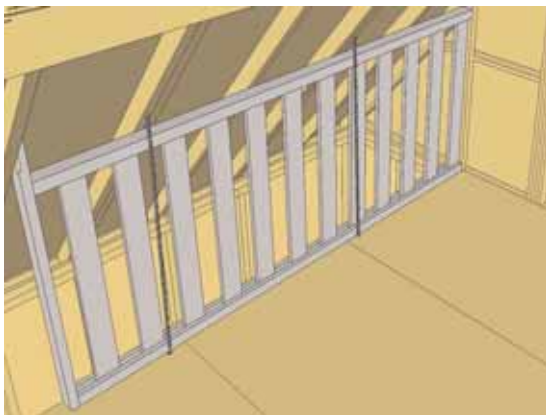
Completed Safety Railing
