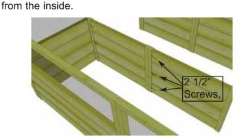
**11.** Align and attach framing of (Part DDD) and (DD Panels) as per Steps 9 & 10. Angle screw panels together with 3 - 2 1/2" Screws from the inside.
