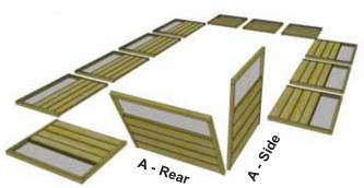
2. Starting in rear corner, position Rear and Side Panels (Part A) - 46" wide together so framing is flush at top and sides. When aligned, attach frames together at top with 1 - 2 1/2" Screw. Use Wood Clamp to hold frames together. Pre-drill rear frame first with 1/8" diameter bit to prevent wood from splitting.
