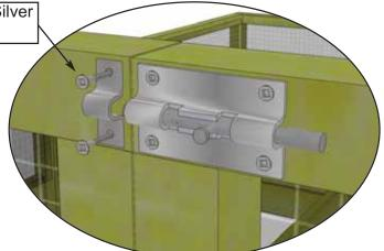
**27.** Attach Barrel Bolt (male and female pieces) to side framing of trellis/screen. Use 6 - 3/4" Silver screws.
