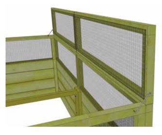
**26.** Lift trellis/screen into the up position. Screw male portion of **Eye Hook** into trellis/screen side framing and female piece into side framing of side wall. Do a dry run first to confirm correct position. Complete both sides.
