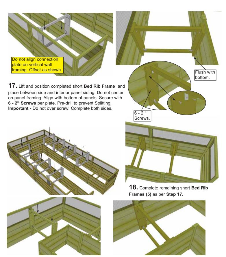
**19.** Lift and center completed longer **Bed Rib Frame** on rear and end interior panels. Align with bottom of panels. Secure with **6 - 2" Screws** per plate. **Important -** Do not over screw!
