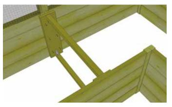
**18.** Lift and center completed longer **Bed Rib Frame** on rear and end interior panels. Align with bottom of panels. Secure with **6 - 2**" **Screws** per plate. **Important -** Do not over screw!
