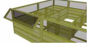
**24.** Complete attachments of both back wall trellis/screens to rear wall framing. Confirm screens can move up and down smoothly. Adjust if necessary.
