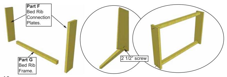
13. To complete rib assembly, locate all 10 Bed Rib Connection Plates (Part F) - 1" x 5 1/2" x 20".
