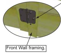
**21.** Attach **Black Barrel Bolt** (male and female pieces) to door and front wall panel frame with **6 - 3/4" Black Headed Screws.** Pre-drill first to prevent wood from splitting. Do a dry run first to confirm fit
