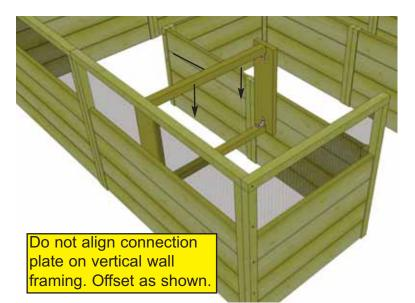
**16.** Lift and position completed short **Bed Rib Frame** and place between side and interior panel siding. Do not center on panel framing. Align with bottom of panels. Secure with **6 - 2'' Screws** per plate. Pre-drill to prevent Splitting. **Important -** Do not over screw! Complete both sides.
