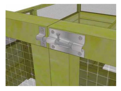
**26.** Attach **Barrel Bolt** (male and female pieces) to side framing of trellis/screen. Use **6 - 3/4**" **Silver screws.** Pre-drill shallow hole first to prevent wood from splitting. Do a dry run first to confirm correct position. Barrel Bolt may be silver/black.
