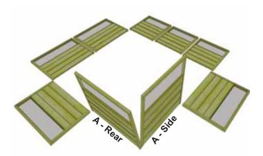
2. Starting in rear corner, position Rear and Side Panels (Part A) - 46" wide together so framing is flush at top and sides. When aligned, attach frames together at top with 1 - 2 1/2" Screw. Use Wood Clamp to hold frames together. Pre-drill rear frame first with 1/8" diameter bit to prevent wood from splitting.
