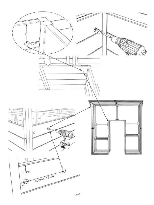
**Step 3** – Start with the interior panel first, with a ¾" Space Bit, drill 4" down and 2 3/8" from the end. Now drill the outside panel holes following the illustration above. One hole will be drilled 1" from the inside of the 2x2 frame and second is approximately 18 ¾" from that mark. Hole location is important so mark holes first with a pencil and then hold the timer assembly up to confirm.
