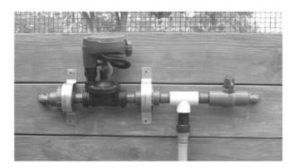
**Step 5 –** The long hose will feed through the other ¾" hole on the inside panel. Long hose may need to be cut shorter so it extends 1" past inside panel. Attach 90 degree elbow with hose nipple to each blue hose end on the inside. See picture below.
