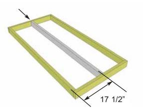
**1.** Floor Joist Frames require one interior Floor Joist attachment each. Center Floor Joist (17 1/2" from outside of Frame to center of Floor Joist) and attach with 2 - 2 1/2" screws per end. You can find the Square Drive Bit for the screws in with the Hardware Kit Bag.
