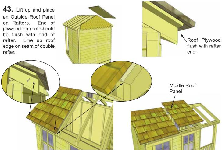
**44.** Place Outside Roof Panel so it sits flush on 3rd rafter from the outside (doubled up rafter). Plywood on roof should be flush with end of rafter at bottom. From the outside, screw down through bottom row of shingles into rafter with 1 - 2 1/2" screw. Angle a 2 1/2" screw from outside rafter into roof plywood. Locate **Middle Roof Panel** and position on Rafters.
