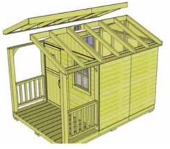
**36.** Place second completed Rafter Section on Gable Walls and position as per **Steps 32 - 34**.
