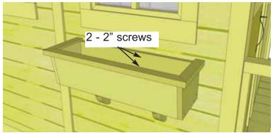
**69**. Assemble Flower Box Kit. Assembly Instructions found in separate manual included. Position completed Flower Box below bottom of window trim and secure with 2 - 2" screws per box. Screw from inside of box into the center wall stud. Attach second screw 2" underneath first screw and once again into the wall stud. Install Flower Box Kits underneath each window.
