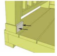
**58.** Attach **Post Base Trims** to bottom of Porch Posts. Attach with 1 1/2" finishing nails. Center a **Rail Support Block** (1 1/2" x 3 1/2" x 3 1/2") under each Handrail Section and secure from top down with 2 - 2 1/2" screws. Complete each Handrail Section.
