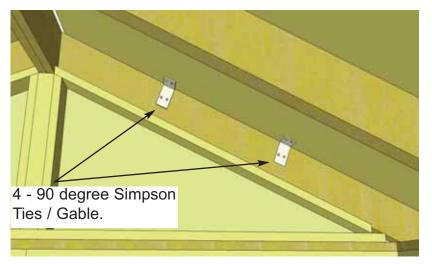
**51.** Position Simpson Strong ties on plywood and outside rafters of back gable and secure with 4 - 1 1/4" screws. There are 4 ties in total.
