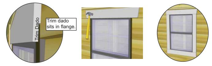
**12.** Starting at rear corner, position a **Wall Panel** on top of plywood floor. Depending on your preference, you may use a **Solid** or a **Window Wall Panel** in this position. If using a Solid Wall, make sure panel is facing up.
