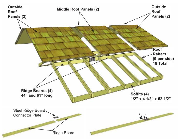
**28.** Locate (1 each) 3/4" x 3 1/2" x 44" & 61" **Ridge Boards** and attach together with **Steel Ridge Board Connector Plates** using 8 - 3/4" screws. Total length when connected is 105". Complete two sets.
