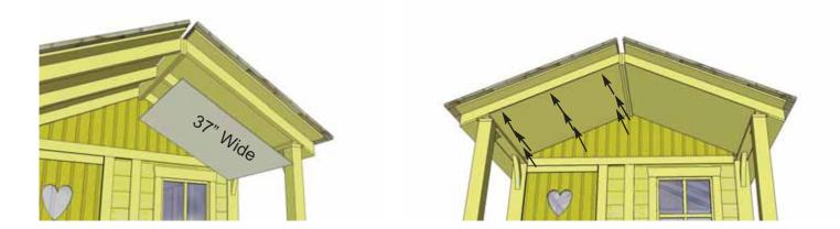
**53**. Position Porch Veneer with best face exposed, flush with front Rafter and Ridge Board. When correctly in place, nail veneer to rafters with 12 finishing nails. Complete both sides.
