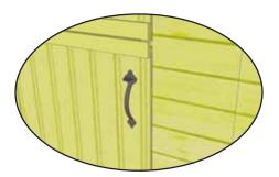
**19.** Attach **Door Handle** and **Interior Silver Barrel Bolt** Hardware. Use 3/4" Black Headed Screws to secure the Door Handle. **Important:** Drill shallow Pilot Holes to prevent wood from splitting. Align male and female Barrel Bolt to Door Framing. Attach with 3/4" Black Headed Screws.
