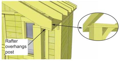
**35.** Rafter will overhang Porch Post when correctly positioned on walls.
