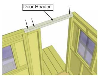
**16.** Attach the **Left Side Door Jamb** to Left Side Wall Stud. Make sure Door Jamb is flush with floor and flush with existing wall stud. Use 3 - 2 1/2" screws to secure. Next, attach the **Door Header** to Door Jamb and Top Plate of Narrow Wall. Use 3 - 2 1/2" screws to secure. **IMPORTANT:** Check door opening measurement at top and bottom. It should be 23 1/2".
