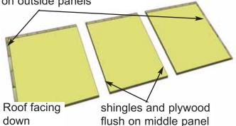
**42.** Identify all **Roof Panels.** There are four **Outside** and two **Middle Roof Panels.** Outside Panels will have shingles overhanging the plywood on one end.
