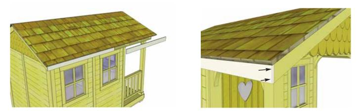
**64.** Attach **Side Facia** to Roof Rafter Ends. There are two Side Facia pieces per side. Secure with 8 - 1 1/2" finishing Nails per piece.
