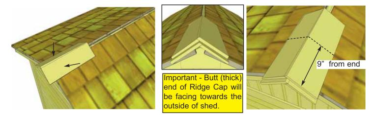
**65.** Place First Roof Ridge Cap on roof peak overhanging shingles by approximately 2". Attach with 2 - 1 1/2" Shingle Nails 9" from end. Place 2nd Ridge Cap 1" back from 1st cap. Attach with 2 - 1 1/2" Shingle Nails 9" from end.
