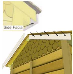
**63**. Attach Facia/Roof Nailing Strips to the underside edge of the plywood roof. Center and attach with 3 - 1 1/4" screws. Complete all four sides.
