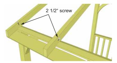
**40.** Attach Rafters in porch area into Top Plate of porch with 1 - 2 1/2" screw per Rafter. Once again, measure 70" from inside of wall plate to wall plate for correct Rafter alignment prior to attaching. **Drill pilot holes in rafters on angle first to prevent splitting and then screw down.**
