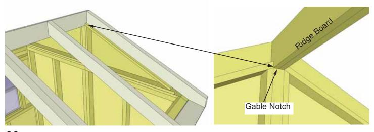
**33.** Slide Rafter Section up on Gable Framing until bottom of Ridge Board slips into Gable Notch.
