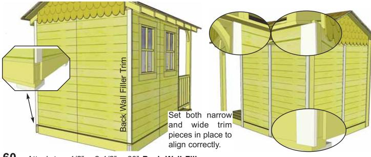
**60.** Attach two 1/2" x 2 1/2" x 60" **Back Wall Filler Trims** to back wall corners. Hammer with 6 - 1 1/2" finishing nails. Flush trim with skirting and siding.
