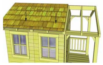
**45.** To confirm, **Middle Roof Panel** will have roof plywood flush with outside of shingles. Place on Middle Rafters and align panel as per **Step 44.** Screw panel down to rafters with 2 - 2 1/2" screws in the bottom row of shingles.
