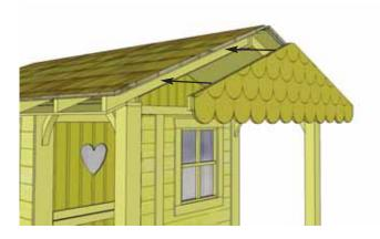
**54.** Attaching the **Decorative Front Gable** is next. Place the Decorative Front Gable underneath porch roof, tight against roof rafter. Be sure to center gable evenly from side to side and place tight up to roof plywood.
