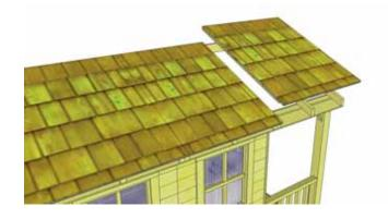
**46.** Lift up, position and attach **Front Outside Roof Panel** on Rafters as per **Step 42- 44**. Continue and place opposite **Rear Outside Roof Panel** on Rafters.
