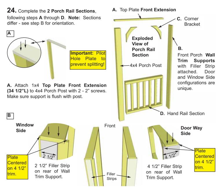
**B.** Attach 1x4 1/2" **Wall Trim/ Supports** to Front Extension using 2 - 2" screws. Make sure Front Extension is Flush to back of wall trim and centered 1/2" on each side. **Note:** there are 2 different wall supports for left & right. See diagram for proper orientation.
