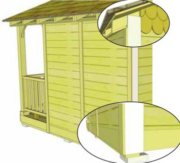
61 Align and attach both Rear and Sidewall Trims (7 @ 1/2" x 2 1/2" x 64") on each wall seam and in each corner. Position tight underneath Soffit and Rafter. Narrow Trims will cap Wide Corner Trims in Rear and side of Porch. See Step 62 for detail. Use 6 - 1 1/2" finishing nails to secure each piece. Note that Narrow Trim will sit slightly below Bottom Skirting when correctly attached. Do a dry run with both Narrow and Wide Trims prior to attaching to confirm positioning.
