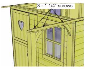
Screw Side Top Plate into porch section with 3 - 1 /4" screws. Screw into Corner Brackets and Post to conceal screws. Complete the other Porch section.
