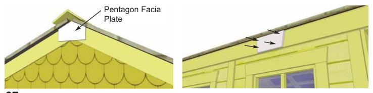
67. Attach Pentagon Facia Plate to Rear and Front Facia with 4 - 1 1/2" finishing nails. Facia Plate will cover any gaps existing where Facia's come together at peak. Attach Facia Detail Plates (2) where Side Trims meet. Use 4 - 1 1/2" finishing nails to secure.
