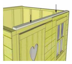
**21**. Position the **Front Top Plate** on top of Door and Front Wall Panel. Front Top Plate is straight cut on the ends and is 70" long. Once again, the Top Plate will be flush with inside of Top Wall Plate. Attach with 4 - 2" screws into Header and Wall Framing.
