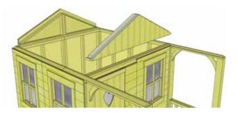
**27.** Position the **Middle Gable Wall** on top of Front Top Plate. When in correct position, attach with 2 - 2" screws as per **Step 26.** Complete installation in **Step 39.**
