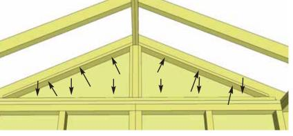
**37.** At the peak, align Ridge Boards so they are flush together and secure them with 12 - 1 1/4" screws. **IMPORTANT:** If there is a gap between Ridge Boards, try pushing Side Walls closer together from outside. Walls should be 70" apart at top from inside of Wall Plate to Wall Plate.
