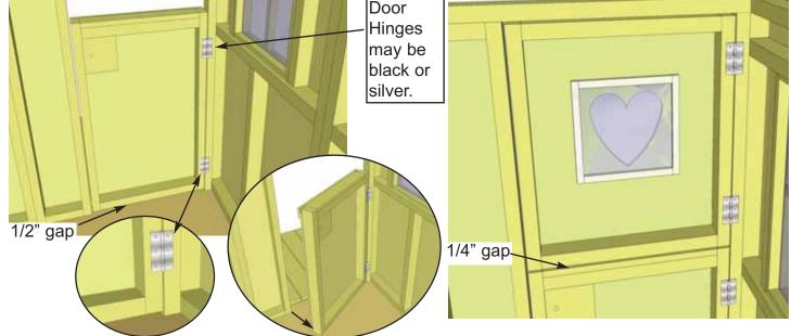
**18.** Attach 2 Hinges (top and bottom) to Bottom Door framing with 3/4" Black Headed Screws. Position the Door into door opening. Leave a 1/2" gap between floor and bottom of door framing. Use Spare Shingle to help shim door into proper position. Initially, secure Door to Door Jamb with one screw per hinge. Check door alignment by moving door back and forth. When satisfied with position, completely secure Door to Door Jamb. Follow same procedure for Top Door leaving 1/4" gap between doors.
