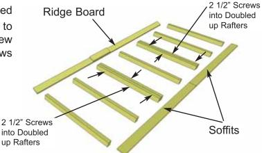
**30.** Attach completed Ridge Board to ends of both outside rafters with 2 - 2" screws per end. Measure and position interior Rafters as illustrated below. When positioned correctly, attach Ridge Board to remaining rafters with 2 - 2" screws /rafter end.
