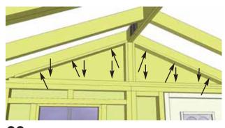
**39.** Secure Rafters to Middle Gable Wall framing and Top Wall Plates with 12 - 2" screws.
