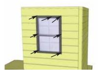
**11a.** Position Window Trim around window doing a dry run first and attach with  $4 - 1 \frac{1}{2}$  finishing nails per piece. The window kit trim pack =  $1x \frac{24 \frac{1}{16}}{1} = \frac{10}{3} \times \frac{23}{2} = \frac{1}{3}$  sides and bottom. Window trim has a small dado on reverse face. Outside flange of window will roughly sit in the dado to give a better fit.
