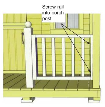
**57.** Toe-nail or angle screw all Porch Posts to floor with 3 - 2 1/2 screws per post. Drill pilot holes to avoid splitting posts. Position Screws so Post Base Trims in **Step 58** will cover. Confirm Porch Post alignment as per **Step 25** prior to attaching.
