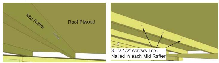
**52.** To further secure roof panels, from the inside, drill pilot holes in each Mid Rafter (3 per Rafter) on an angle. Using 3 - 2 1/2" screws, secure rafters to roof plywood. **Note:** from outside, have a helper push roof panel down so plywood sits flush against rafter when securing. In Porch area, angle screw both the mid and outside rafters.
