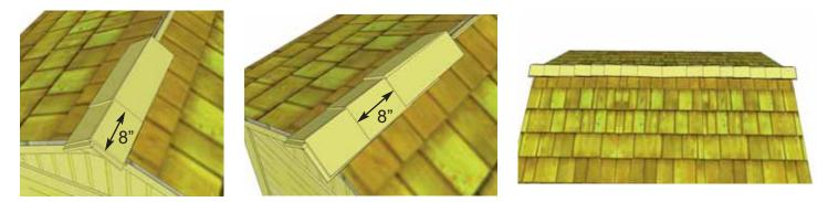
**66.** Place 3rd Ridge Cap 8" back from 2nd (enough to cover shingle nails). Attach 3rd Ridge Cap down as per **Step 65.** Continue to position and attach Ridge Caps until half the roof is complete. From opposite side, position and attach Ridge Caps as described above. Score/cut 1 Ridge Cap to 12" or to fit in the center of roof. Attach center cap with 4 - 1 1/2" Shingle Nails.
