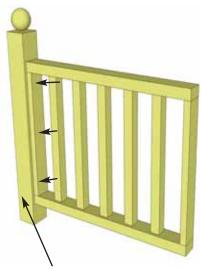
Use Rail Support Block (3 1/2" high) from bottom of post to align rail. Attach rail to post with 3 - 2" screws.
