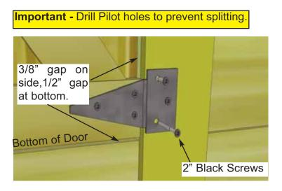
**63.** Now secure the Double Doors. Starting with **Right Side Door**, position so there is a 1/2" gap on bottom, and approximately 3/8" on the side. Use a spare piece of siding or shingle to shim door in place at the bottom. Using 2" black screws, secure bottom hinge to Door Trim. **Hint:** Do not attach all the 2" screws until both doors are positioned correctly. You can use a Screw Driver to tighten screws completely so you don't over tighten.
