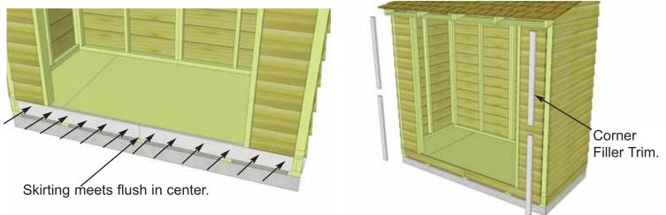
**50.** Use 6 nails on front skirting piece where doors will be installed. This ads extra support to a high traffic area.
