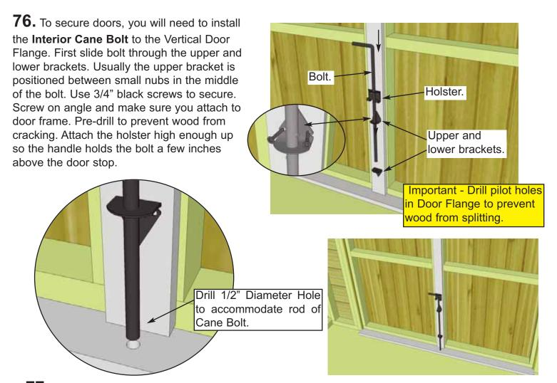
**77.** Once the Cane Bolt is attached, close doors and mark a hole in the stop to accommodate the bolt. You can bang the top of the bolt using a hammer and a block of wood to prevent damage. Once complete, open doors and drill hole where previously marked with 1/2" bit.
