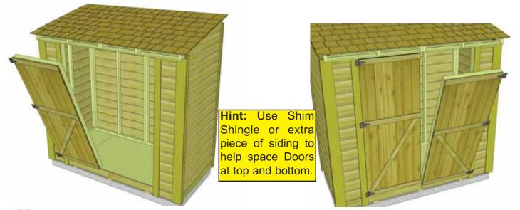
**62.** With Hinges attached, position doors in opening. You will need some assistance to hold doors in place.
