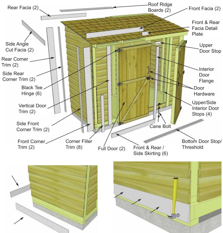
**47.** Attach **Bottom Skirting** (3/4" x 4 1/2" x 45 1/4" - bevel) around the base of the shed. Skirting will hide floor framing. Start with side skirting pieces first and attach with 4 - 1 1/2" finishing nails per piece.
