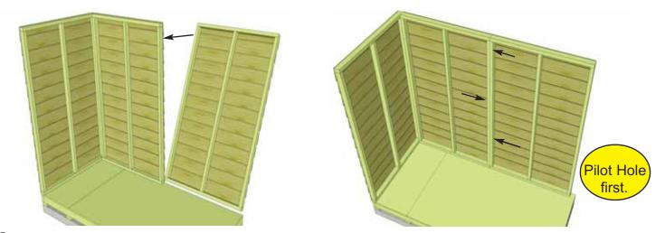
**13.** With the corner wall attachment complete, position the second rear wall panel in place so bottom 2x3 wall framing is sitting flush with outside floor framing. Wall siding should overhang floor by approximately 3/4". When positioned correctly, attach both wall panel studs together as per **Step 12** with 3 - 2 1/2" screws.
