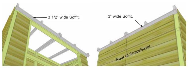
**34.** When Rafter Section is positioned correctly, both Front and Rear Soffits will sit approximately 1/8" away from wall siding. This can vary slightly.
