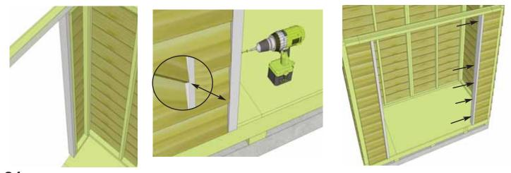
**21.** Locate both **Vertical Door Jambs** (1 1/2" x 3 1/2" x 73") and position flush against front narrow wall stud. The Jamb will sit flush to outside of wall siding. When positioned correctly, secure Jamb using 6 - 2 1/2" screws. Complete both sides.
