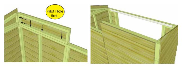
**27.** With 2x3 wall framing aligned, attach Wall Extendor to both the Angled Wall Extendor framing and the rear wall framing with  $5 - 2 \frac{1}{2}$  screws.
