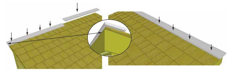
**69.** Position first **Roof Ridge Board**  $(1/2" \times 4 1/2" \times 51 5/8")$  at the rear of roof to cap off shingles and facia. Ridge Boards should meet on seam of roof panels. When aligned correctly, attach with 4 - 1 1/2" nails per piece.
