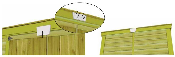
**70.** Attach Facia / Detail Plates to cover seams where Front and Rear Facia pieces come together. Secure with 4 - 1 1/2" finishing nails per piece.
