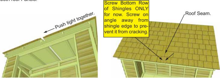
**40.** With Roof Panels aligned, screw panels down to center rafters with 2 - 2 1/2" screws in **Bottom** Row of Shingles Only (1 screw per panel).
