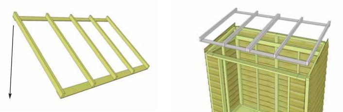
**32.** Carefully flip completed Rafter Section over so 3 1/2" wide Soffit is facing the front and place on SpaceSaver walls. **Note:** once again, make sure 3 1/2" wide Soffit is positioned to the front of the shed.
