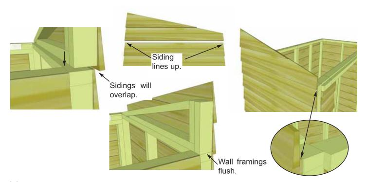
**23.** Align wall framing of Angled Wall Extendor and Side Wall so they are flush at the back. The siding for both walls should also align evenly from front to back.
