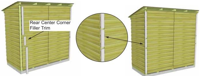
**53.** Position and attach Corner Filler Trims in the rear as per **Step 52.** There is an additional 10" long **Rear Center Corner Filler Trim** that you will need to center and attach as well using 2 - 1 1/2" nails.
