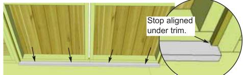
74. Attach Lower Door Stop /Floor Threshold (3/4" x 2 1/2" x 64") between door jambs. Check door alignment first and then attach with 4 - 1 1/4" screws. Optional - caulk the lower edge of threshold to prevent water penetration.
