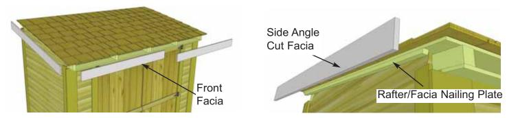
**66.** Locate and identify all Facia pieces: **Front & Rear Facia (4)** (1/2" x 4" x 50 1/2"). **Side Angle Cut Facia (2)** (1/2" x 4" x 54 1/8"). In front corner, align side and front Facia together.
