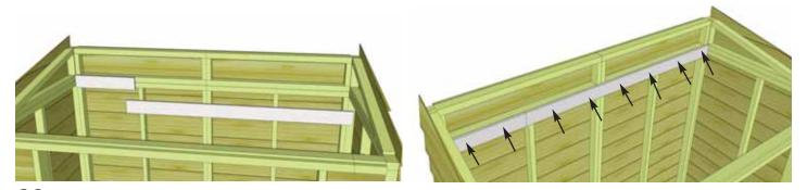
**29.** Attach Horizontal Wall Cleats (1 @ 3/4" x 3 1/2" x 70", 1 @ 3/4" x 3 1/2" x 21") to Wall Extendor bottom framing and Rear Wall top framing, so that cleat is flush with extendor framing. There is a short and a long wall cleat. Alternate alignment of screws, so half screw into Wall Extendor Framing and half into Rear Wall Top Framing. Use 8 - 1 1/4" screws.
