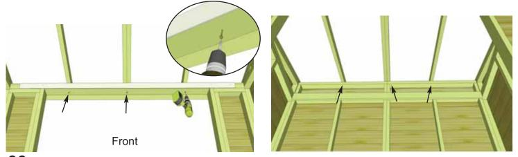
**36.** With outside rafters properly secured, completely secure remaining interior rafters using 6 - 2 1/2" Screws. Screw into rafters from inside of Header on an angle at front of shed, and from inside of Extension Wall Framing at rear of shed.
