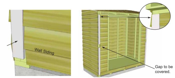
**52.** Attach **Corner Filler Trims** where gaps exist in front corners (2 per side). Hammer with 8 - 1 1/2" finishing nails. Position bottom filler just below wall siding. Top filler just below soffit. Gap in middle.
