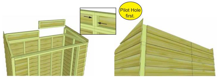
**28.** Position and secure 2nd Wall Extendor Panel as per **Steps 26 & 27**. Additionally, attach to first Extendor with 2 - 2 1/2" screws.
