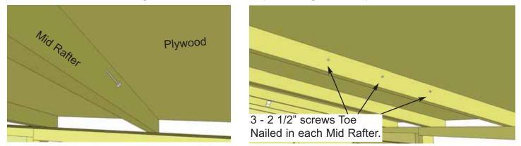
**46.** To further secure roof panels from the inside, drill pilot holes on an angle in each panel's Mid Rafter (3 per Rafter). Using 3 - 2 1/2" screws, secure rafters to plywood.
