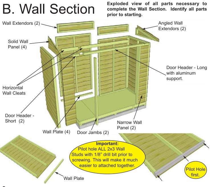
**9.** Locate 4 **Solid Wall Panels** and 4 **Wall Plates** (1 1/2" x 2 1/2" x 45 1/2"). Attach Plates to bottom of studs of each wall panel with 3 - 2 1/2" screws. Position so plates are flush with framing.
