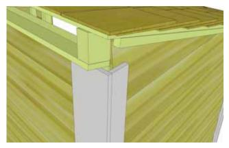
**58.** To completely trim out rear corners, locate **Side Rear Corner Trims** (1/2" x 2 1/2" x 88 3/4") and **Rear Corner Trims** (1/2" x 5 1/2" x 88 3/4"). Align and attach as per **Step 57**.
