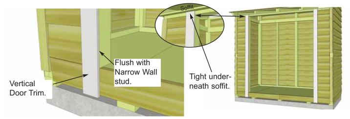
**54.** Locate Vertical Door Trim  $(2 - 1/2" \times 3 1/2" \times 79")$ . Position Door Trim flush with outside of narrow wall stud. Trim should be aligned tight underneath Soffit. Attach with 8 - 1 1/2" finishing nails.
