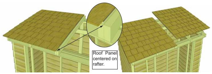
**39.** For correct Roof Panel position, align panel so plywood sits evenly on Center Rafters. Complete both roof Panels.
