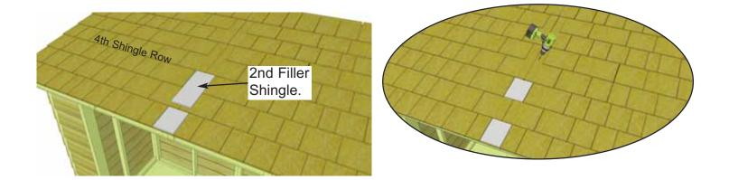
**43.** Slide 2nd **Filler Shingle** up and underneath fourth shingle row. Follow **Steps 41 - 42** to align and attach.
