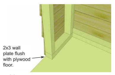
**16.** Once again position the 2x3 wall plate so it sits flush on floor and siding overhangs. **Note:** Narrow Wall Panel is only 73" high.
