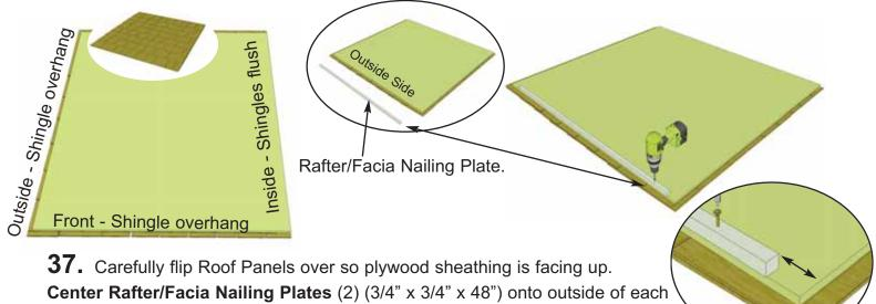
**Center Rafter/Facia Nailing Plates** (2) (3/4" x 3/4" x 48") onto outside of each panel flush with plywood. Attach with 4 - 1 1/4" screws evenly spaced. The Rafter/Facia Nailing Plate provides for a greater nailing surface later when you attach side facia.
