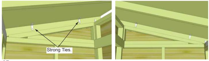
**45.** Secure roof panels to walls at both ends by positioning 2 Simpson Strong Ties on plywood and outside rafters and securing with 2 - 1 1/4" screws per Strong Tie. Complete both sides.
