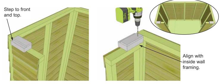
**19.** Locate both **Door Headers - Short** (step facing up and out). Attach both short end pieces using 2 - 2 1/2" screws per piece. Screw from top down into wall framing. Align to inside of wall framing and tight against side wall.
