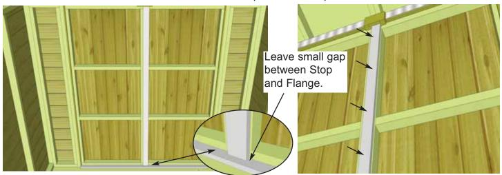
**75.** Position and attach Interior Vertical Door Flange (1/2" x 2 1/2" x 70") on inside door frame (left door from outside/right from the inside) using 6 - 1 1/4" screws. Position on inside edge of left door frame so Flange overlaps right door frame by about 3/4".
