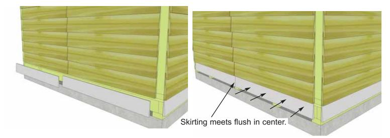
**48.** Rear skirting pieces will meet together in the center. Secure with 4 - 1 1/2" finishing nails per piece.
