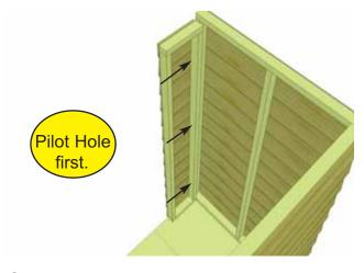
**17.** When correctly positioned, secure Narrow Wall Stud to Side Wall Stud with 3 - 2 1/2" screws.
