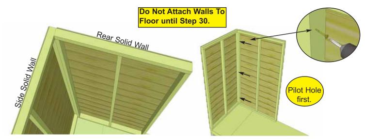
**12.** Butt both vertical wall studs of side and rear walls together and attach with 3 - 2 1/2" screws. Screw at the bottom, middle and top of stud to secure properly. Have helper push wall framing together while securing to ensure tight fit. **Note: Drill pilot holes in studs to prevent splitting**.
