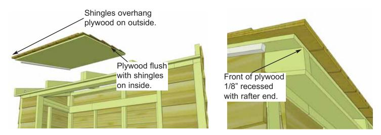
**38.** Correctly orientate Left Side Roof Panel, with shingles overhanging plywood on the side of the shed and flush with plywood to the middle. Place on rafters with front of plywood just about flush with rafter ends but just slightly recessed. Doing so allows front facia to sit better.
