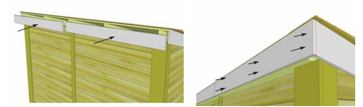
**68.** Place and align rear and side facia for best possible fit with rear caping side facia. Attach facia to rafter ends with 6 - 1 1/2" finishing nails per piece. Complete both rear facia pieces.
