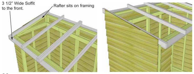
**33.** Position completed Rafter Section on top of walls. Outside Rafters will sit on Extension Wall framing and be positioned equally from side to side.
