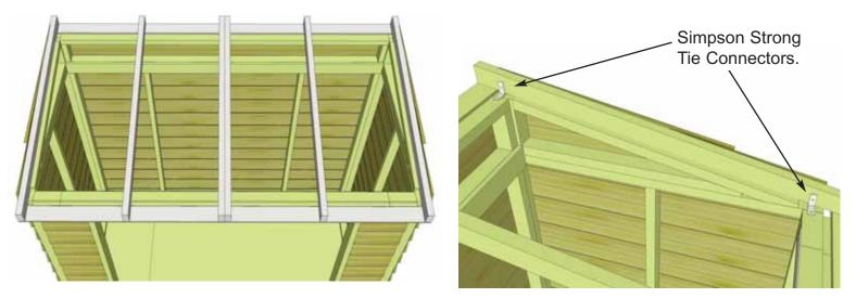
**35.** With Rafter Section correctly aligned, secure rafters to walls using **Simpson Strong Tie Connectors**. Start with outside rafters and secure 2 Strong Ties with 1 1/4" screws. Screw into Wall Extension Framing at the rear and Wall Panel top framing at the front. Complete both sides.
