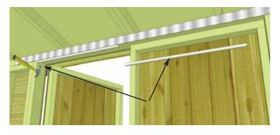
**71.** Attach **Upper Interior Door Trim (2)**  $(1/2" \times 1/2" \times 28 7/8")$  positioning 1st trim against door jamb and underneath door header flush to edges on inside as shown to the right. Attach with 4 - 1 1/2" finishing nails.
