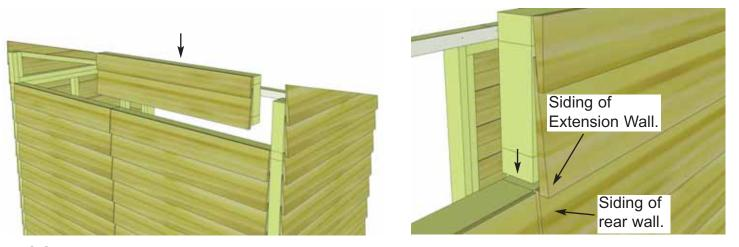
**26.** Locate one **Wall Extendor** and place on rear wall panel with siding of extendor overlapping that of the rear wall.
