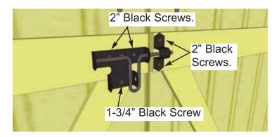
**79.** Attach Black Barrel Bolt as illustrated above with 2" & 3/4" Black Screws. Note how female part of Barrel Bolt is positioned higher than male. Do a dry run first to position Barrel Bolt correctly. **Important** - Drill pilot holes with 1/8" drill bit prior to securing with screws to prevent wood splitting. On 3/4" screw, drill shallow pilot hole only.
