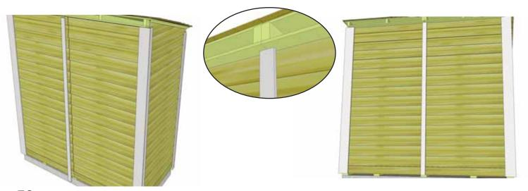
**59.** Attach **Rear Middle Trim** (1/2" x 2 1/2" x 88 3/4") where wall panels come together at rear seam. Attach with 8 - 1 1/2" finishing nails aligning tight underneath soffit and center on seam.
