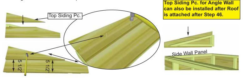
**22.** Locate an **Angled Wall Extendor** and **Top Siding Piece for Angled Wall Extendor (L/R)**. Position top siding on wall extendor and align as shown above. Attach with 3 - 1 1/2" finishing nails to top wall framing. There are left/right top siding pieces. Use rough surface side out.. Place finished wall extendor on side wall panel frame. Complete both sides now. **Note:** Bottom siding of wall extendor will overhang and cover siding of side wall.
