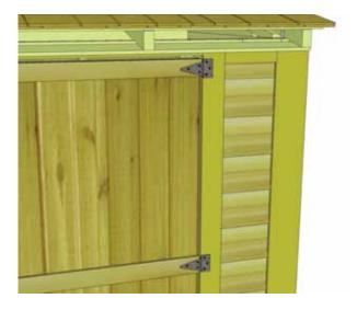
**64.** Make sure Door Panel is aligned evenly at top and edge. When aligned correctly, attach top and middle hinges to narrow trim with 2" black screws.
