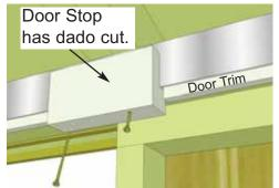
73. Attach Upper Door Stop dado cut (1 1/2" x 2 1/2" x 6") underneath door header with 2 - 2 1/2 screws. Stop is pre-drilled on angle. Evenly space between trim.
