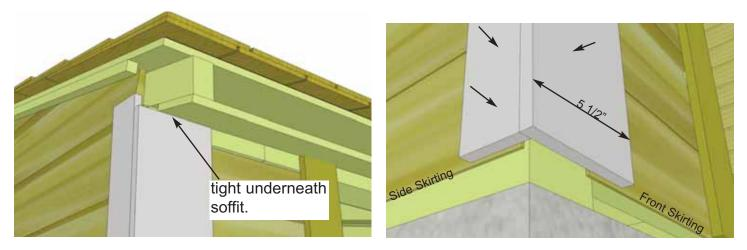
**57.** Place both trims in front corner and align as illustrated above. Do a dry run prior to attaching to achieve best fit. Start with 5 1/2" wide Front Corner Trim and align tight underneath soffit to determine vertical height. Attach with 8 - 1 1/2" finishing nails per piece. Position and attach Side Front Corner Trim (2 1/2" wide) using 8 - 1 1/2" nails, aligning at bottom with wide trim.
