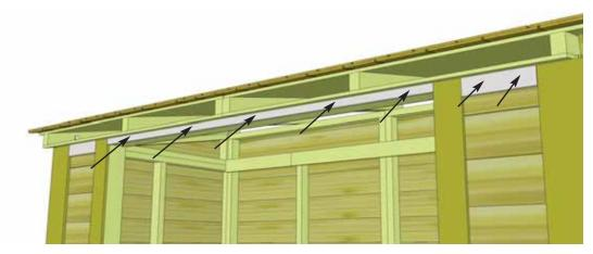
**60.** To trim out door, locate Horizontal Door Trim  $(1/2^{\circ} \times 1 \ 1/4^{\circ} \times 64^{\circ})$  and both Horizontal Narrow Wall Trims  $(1/2^{\circ} \times 2 \ 1/2^{\circ} \times 8 \ 1/2^{\circ})$ . Position as shown above and attach with 1 1/2° finishing nails.
