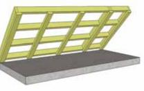
5. With Floor Runners attached, carefully flip the floor over and place on your foundation. Caution - you may need 2 people to assist you. Be careful when laying floor down not to bend or twist floor. Note: The floor will be flipped over and floor runners will sit on your foundation. It is important to note that having a level foundation is critical. Choosing a foundation will vary between regions. Typical foundations can be concrete pads or patio stones positioned underneath the floor runners.
