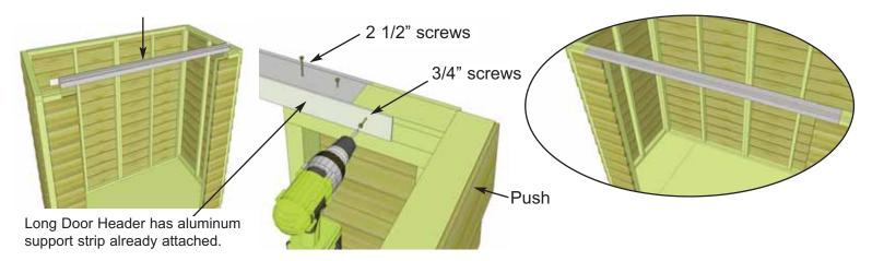
**20.** Locate **Door Header - Long** (2" wide aluminum support attached already). Align step on header facing up and out and with support strip to the inside of shed. Attach using 2 - 2 1/2" screws per end as shown above. **Hint:** Have 2 helpers push Side Walls together to close any gaps between Headers. Complete both sides. Attach support strip to short headers with 2 - 3/4" screws.
