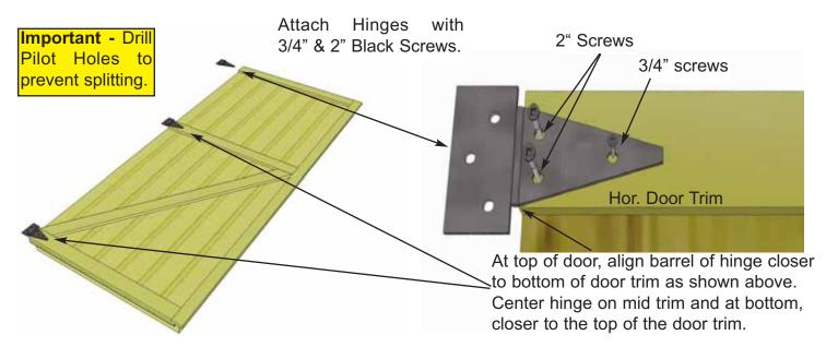
**61.** Attach Door Hinges to both **Left** and **Right Side Double Doors**. Position Hinges equally on door trim as shown above and attach with Black 3/4" and 2" screws.
