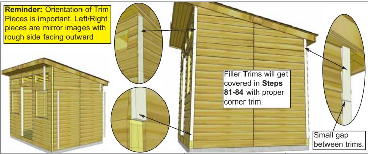
**80.** Position **4R - Filler Trim** (they serve as nailing strips) in corner of side wall, aligned flush with top of bottom skirting. Attach with **4 - 1 1/4" Screws** and repeat for all 4 corners. Next, attach **4S** & **4T - Front/Rear Top Filler Trim** with **2 - 1 1/4" Screws** per piece.
