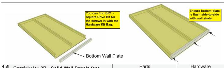
**14.** Carefully lay **2B - Solid Wall Panels** face down. Position and attach **2C - Bottom Wall Plates** to bottom of wall studs of each wall panel with **3 - 2 1/2" Screws**. Position so plates are flush with framing.
