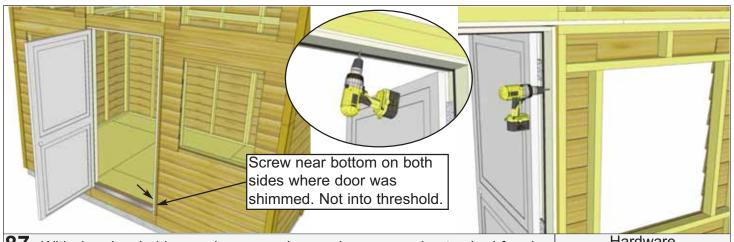
**87.** With door leveled in opening, open door and secure casing to shed framing where you shimmed. Use **2 - 2 1/2" Screws** on top and **3 - 2 1/2" Screws** on each side. Do not screw into threshold.
