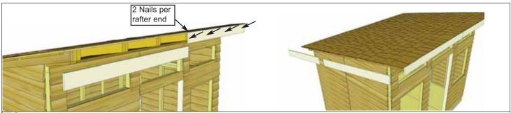
73. Align and attach remaining front facia as per Step 72. Align next two side facias on opposite side as first side facia. Once again, do a dry run before attaching. There will be a Facia Detail Plate attached in Step 76 to hide any gaps where facia pieces meet in the middle.
