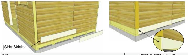
**77.** Attach **40 - Bottom Skirting** around base of the shed. Skirting will hide floor framing. The side skirting pieces will meet together in the center. Gaps on outside will be covered by wide trim pieces later. Start with side skirting pieces first and attach each with **4 - 1 1/2" Finishing Nails**.
