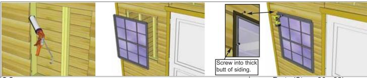
**90.** To reduce possible water from penetrating into the window cavity, caulk gap on both sides of window opening prior to installing the **4AI - Large Window Inserts.** Position insert in cavity and secure with **8 - 1 1/4" Screws**. Make sure to screw insert into the thick butt of the siding only.
