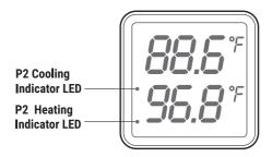
**P2 Heating Indicator LED:** If P2 Temperature Control Function selected heating mode, the indicator LED is on, otherwise off.
