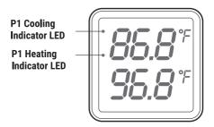
P1 Heating Indicator LED: If P1 Temperature Control Function selected heating mode, the indicator LED is on, otherwise off.
