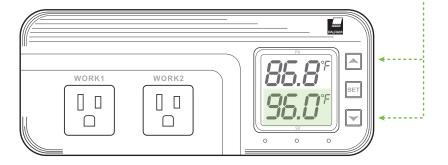
**Shortly press SET button to exit setup mode**
