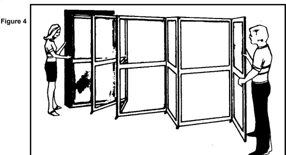
**D)** Align the two wall assembly ends with the vertical **U-Channels (Item 20)** previously attached to the furring, push the wall panels into the **U-Channels (Item 20)** until they are fully inserted and tight against the house.
