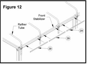
C) Cut the remaining 1" foam (Item 29, used in Figure 1) into strips to fit between the rafters and apply strips to the top of the front wall panels (See Figure 12).
