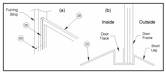
F) Locate the **Threshold(s)** (**Item 23**). The threshold(s) are placed under the doors as shown in **Figure 5b**. Simply lift panel assembly, center thresholds under doors, and allow door frame to slip into the channel in the threshold. Check the rectangle now formed by the panels is square by measuring diagonals (they must be equal).
