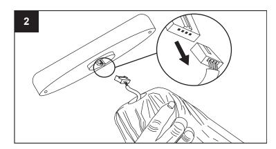
Carefully disconnect the plug from the socket by pressing the tabs surrounding the connection point. Pull apart by holding the plug, never pull on the wires.
