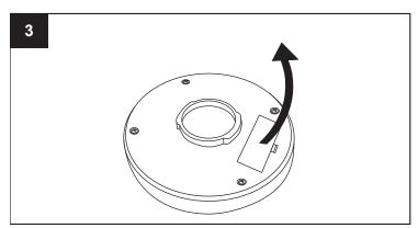
Place the solar panel face-down on a soft, clean surface. Remove the battery housing cover.
