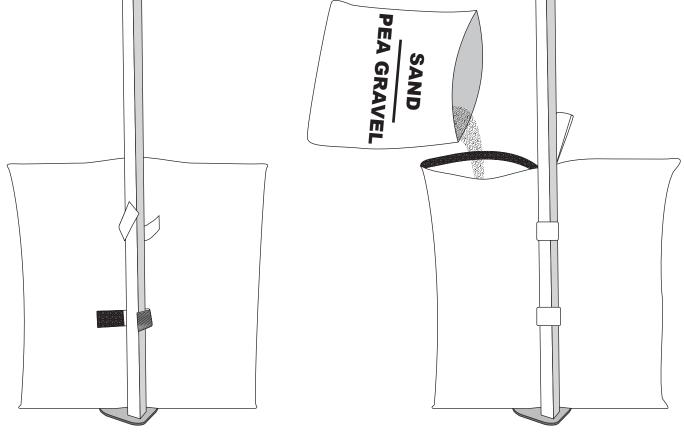
Place the bag on the foot of your canopy. Tightly wrap the hook and loop fastener strips around the canopy leg. Fill both sides of the bag. Do not overfill. Press the hook and loop fastener strips on top of the bag together to close the bag.
