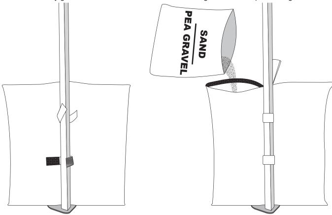
Place the bag on the foot of your canopy. Tightly wrap the hook and loop fastener strips around the canopy leg.
