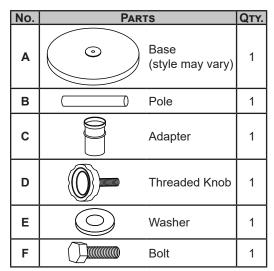
To prevent small parts from being lost during shipping, the washer and bolt are loosely attached to the bottom of the pole. The threaded knob may be inside the pole.
