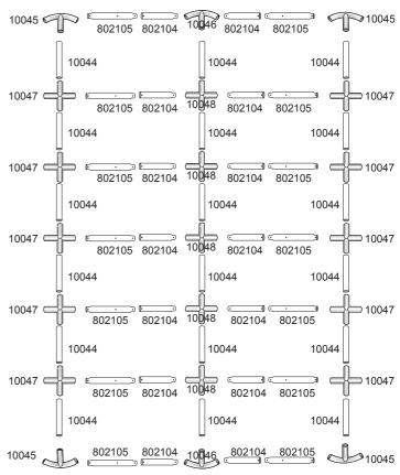
**2. Assemble Roof** Start with center, Fig. 1, using layout shown in diagram above. Bolt roof assembly together as shown in Fig. 1A. Assemble each side of the roof as shown in Fig. 2. Install #802103 truss as shown in Fig. 2A.
