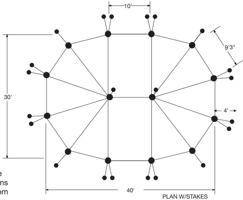
Note: Additional stakes will be necessary in soft soil conditions or whenever stakes pull up from the ground.
