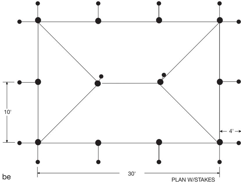
Note: Additional stakes will be necessary in soft soil conditions or whenever stakes pull up from the ground.
