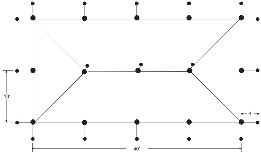
Note: Additional stakes will be necessary in soft soil conditions or whenever stakes pull up from the ground.
