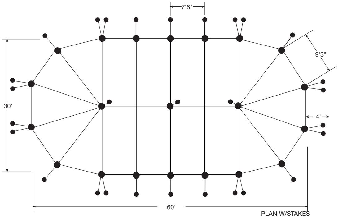
Note: Additional stakes will be necessary in soft soil conditions or whenever stakes pull up from the ground.
