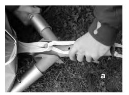
a. With the swivel bracket connected to the frame, hook the small web loop over the metal rod. See above.
