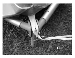
c. Attach the snap pin through the bracket and center arm to secure the corner. See above
